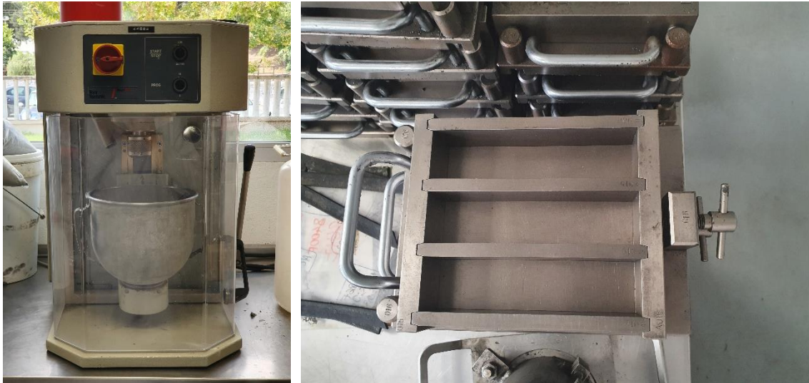
Figure 19 – Blender and mould used in the preparation of mortar samples.
