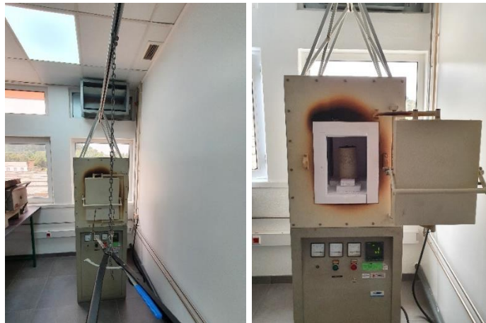
Figure 16 – Muffle furnace used in the production of the amorphous binder.
