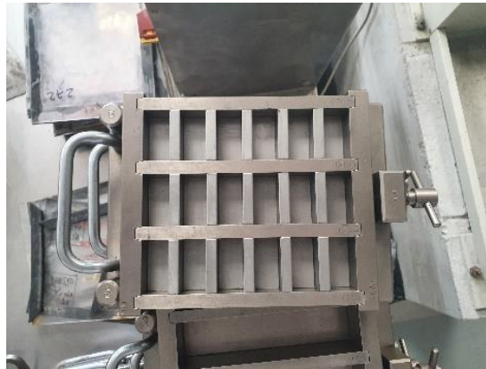
Figure 18 – Mould used in the production of paste samples.
